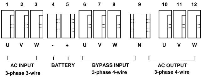
The terminal buses shown are located at the top inside of the 300kVA UPS. Dashed line in each terminal stands for side view of screw holes to tighten lugs.
